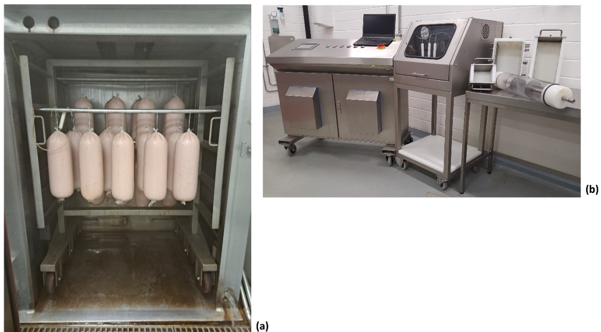
Figure 1. (a) Conventional cooking process of Bologna-style sausages in a steam oven, (b) ohmic heating (OH) plant, consisting of a generator, a datalogger, an OH chamber with three installed PT-100 thermocouples, and various OH cells (from left to right). The OH cell used was the cylindrical-shaped cell (front left).
