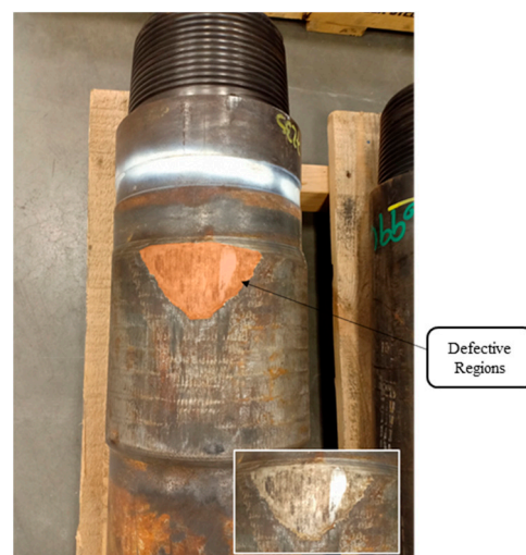
Figure 14. The actual damaged sample repaired via a laser-cladding process.
