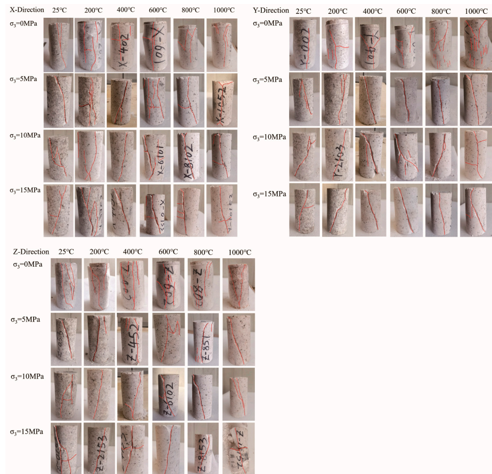
Figure 17. Failure morphology of granite in different sampling directions.
