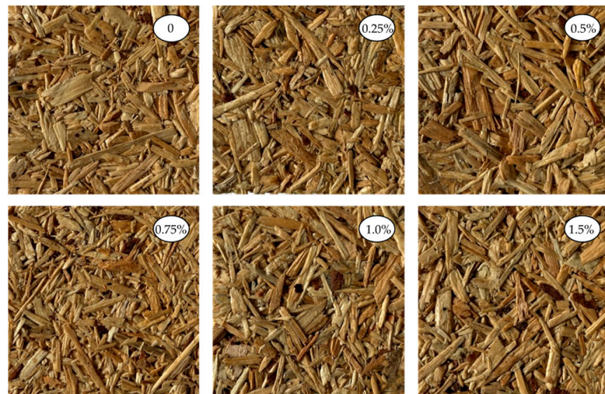
Figure 3. Appearance of the laboratory-made particleboards bonded with UF adhesive modified with ACCS.
