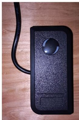
**Figure 3.** Universal reader—LF-band RFID and HF-band RFID.
