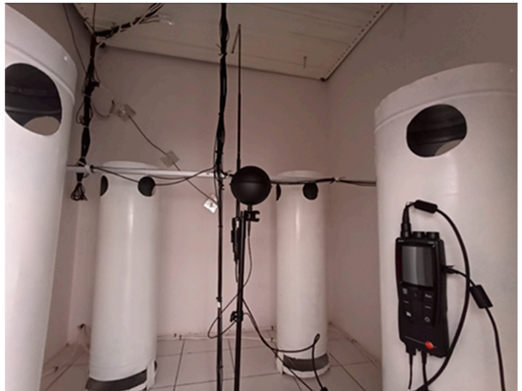
Figure 8. A layout view of the temperature sensors.
