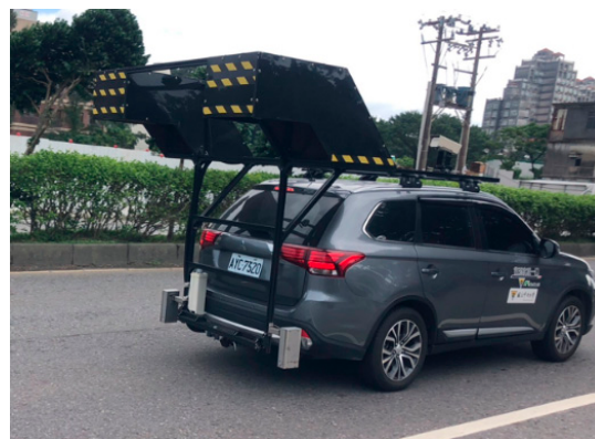
Figure 4. Automated Pavement Inspection Vehicle.
