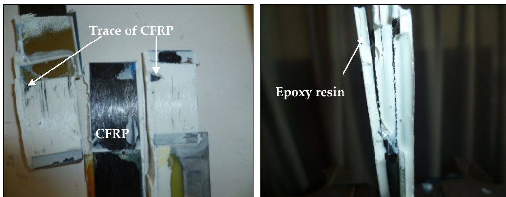
Figure 9. Resin–CFRP rupture type.
