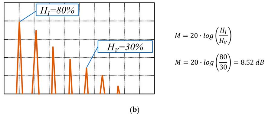
**Figure 6.** Example view of the defectoscope screen. (a) Real image; 1, initial pulse; 2, gain of signal; 3, pulse height read automatically from the measuring gate (5); 4, first pulse ( $H_I$ ). (b) The principle of making measurements with the demonstration of the ultrasonic signal waveform.
