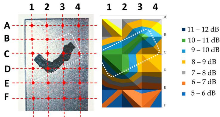
Figure 11. View of a sample after rupture, along with a map showing the value of the ultrasonic measure; the dashed line marks the characteristic area.
