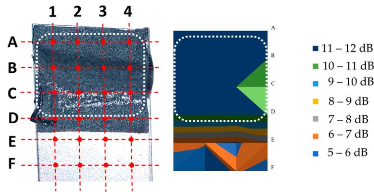
Figure 12. View of a sample after rupture, along with a map showing the value of the ultrasonic measure; the dashed line marks the characteristic area.
