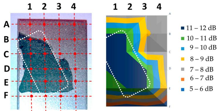
**Figure 9.** View of a sample after rupture, along with a map showing the value of the ultrasonic measure; the dashed line marks the characteristic area.
