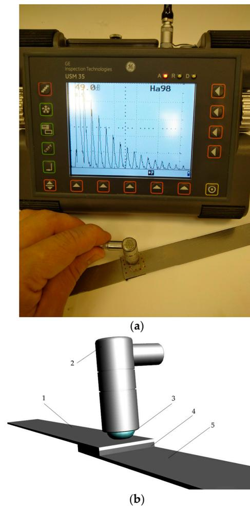
**Figure 4.** Measurement stand: (a) general view, (b) sample and probe model; 1, metal sheet; 2, ultrasonic probe; 3, flexible membrane, 4, adhesive tape; and 5, metal sheet.
