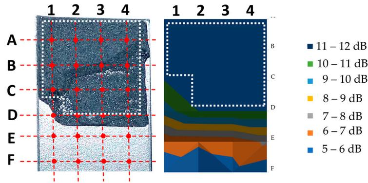
Figure 10. View of a sample after rupture, along with a map showing the value of the ultrasonic measure; the dashed line marks the characteristic area.
