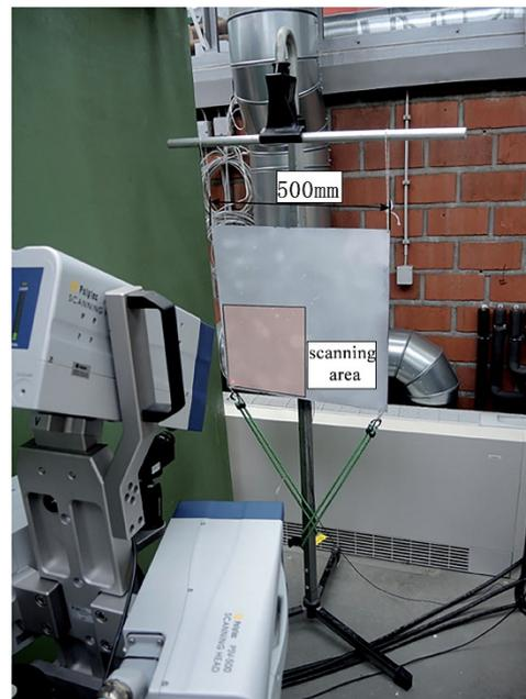
**Figure 31.** Experiment setup for structural plates and laser Doppler vibrometer.
