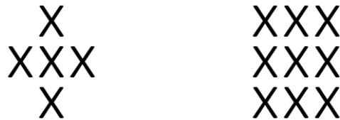
Figure 9. Search locations in Diamond Search (left) and potential search locations in Motion Dynamics Input Search (right).
