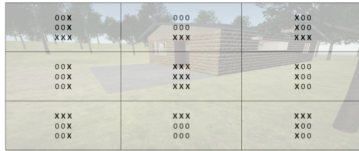
Figure 10. Discrete forward motion search model, depicting selective search patterns based on block positions in an image.
