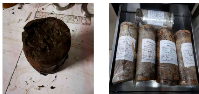
Figure 5. Undisturbed soil specimens collected from site.
