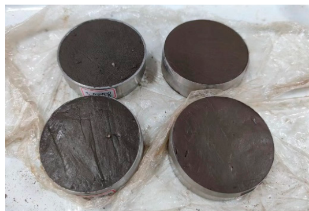
Figure 7. Four specimens prepared for the oedometer test.
