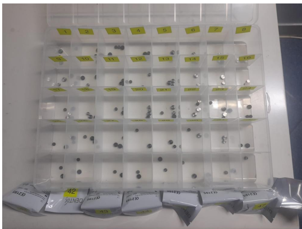
Figure S104. Detail of the storage system for sandblasted probes
