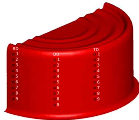
Figure 13. Thickness measurement locations on the sidewall.
