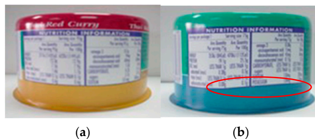
Figure 2. Waving requirement in food can production: (a) accepted; (b) rejected.
