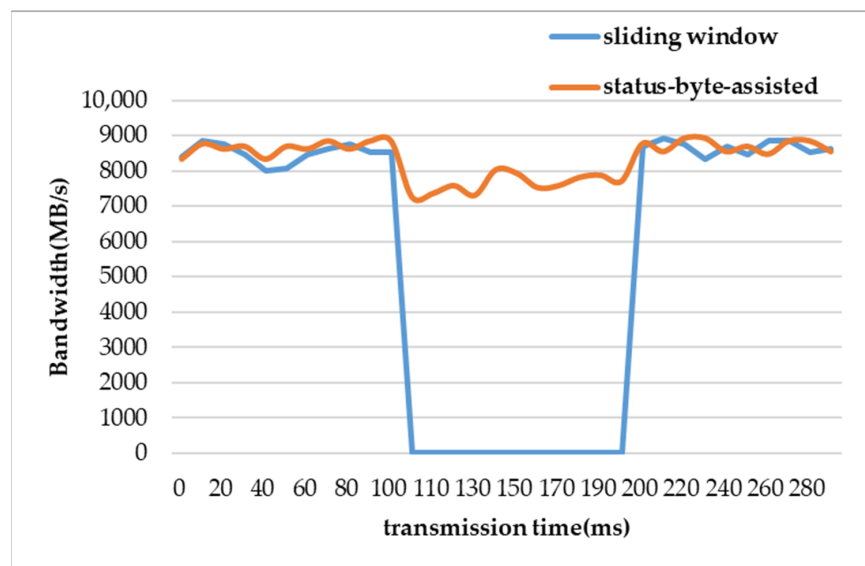
Figure 18. Throughput change in various RDMA transmission mechanisms in response to special demands.
