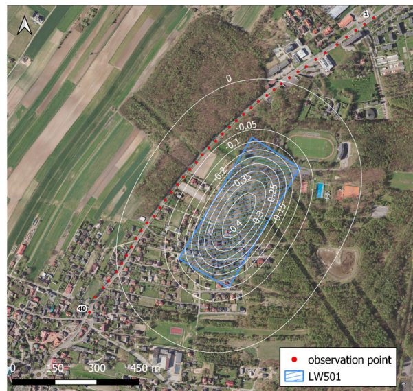
Figure 7. Land surface subsidence (in meters) based on FEM analysis—25 November 2021.
