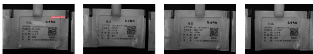
Figure 13. The defect detection results of the original YOLOv8s model. The Chinese characters on the surface of the medicine bag indicate the name of the medicine bag particles and the specific packaging requirements. From the above picture, we can see that the small defects cannot be identified by the original model.
