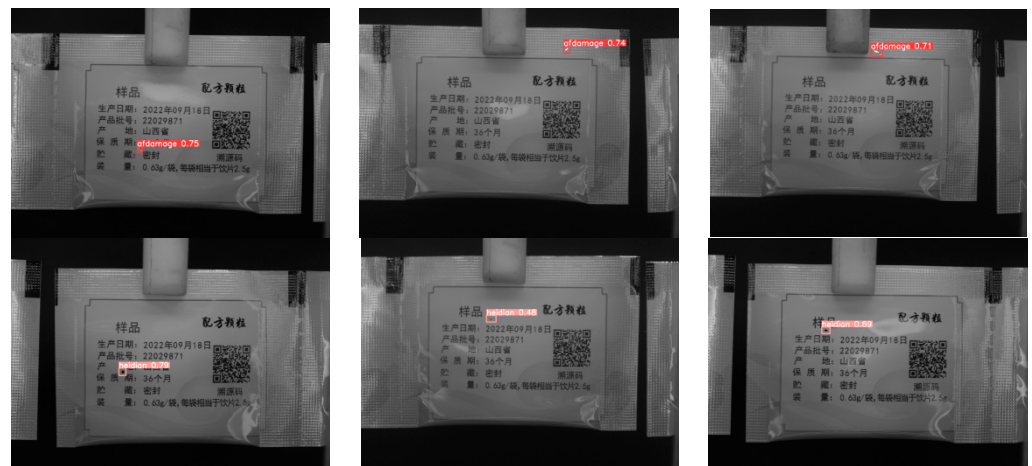
Figure 11. FSNB_YOLOv8 Defect Detection Result Example. The Chinese characters on the surface of the medicine bag indicate the name of the medicine bag particles and the specific packaging requirements. From the above picture, we can see that small defects can be identified by the model.
