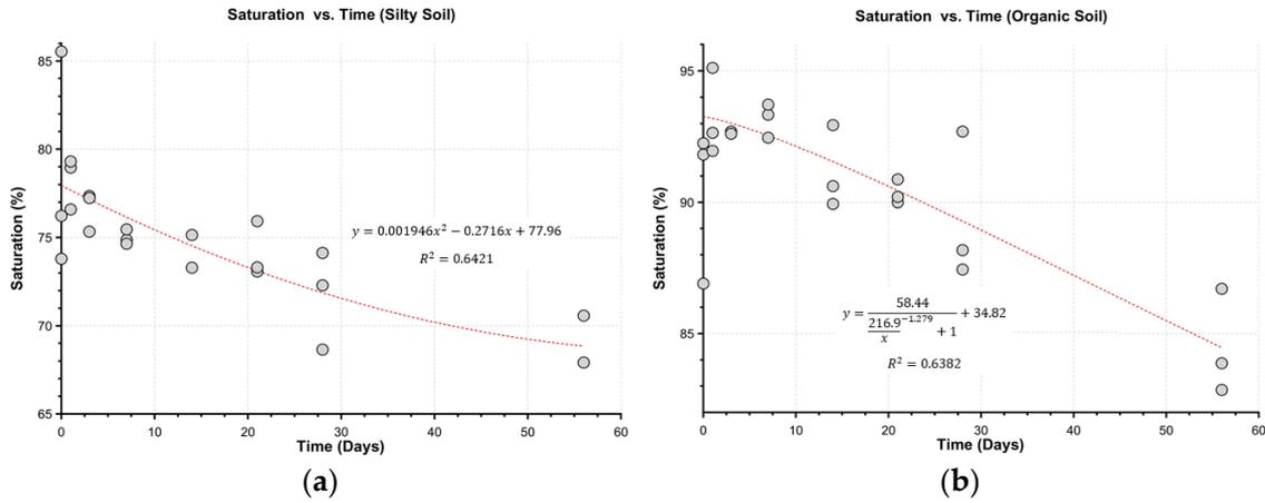
Figure 12. Correlation equation based on test results and elapsed time for the saturation of (a) silt; (b) organic soil.
