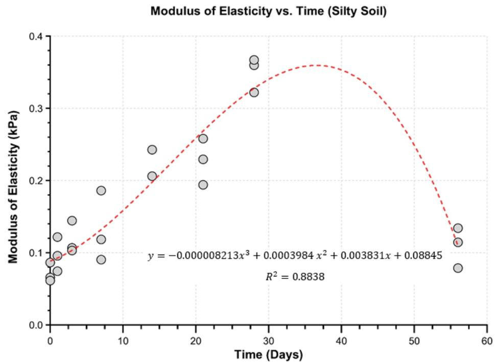
Figure 15. Correlation equation based on test results and elapsed time for the modulus of elasticity-silt.
