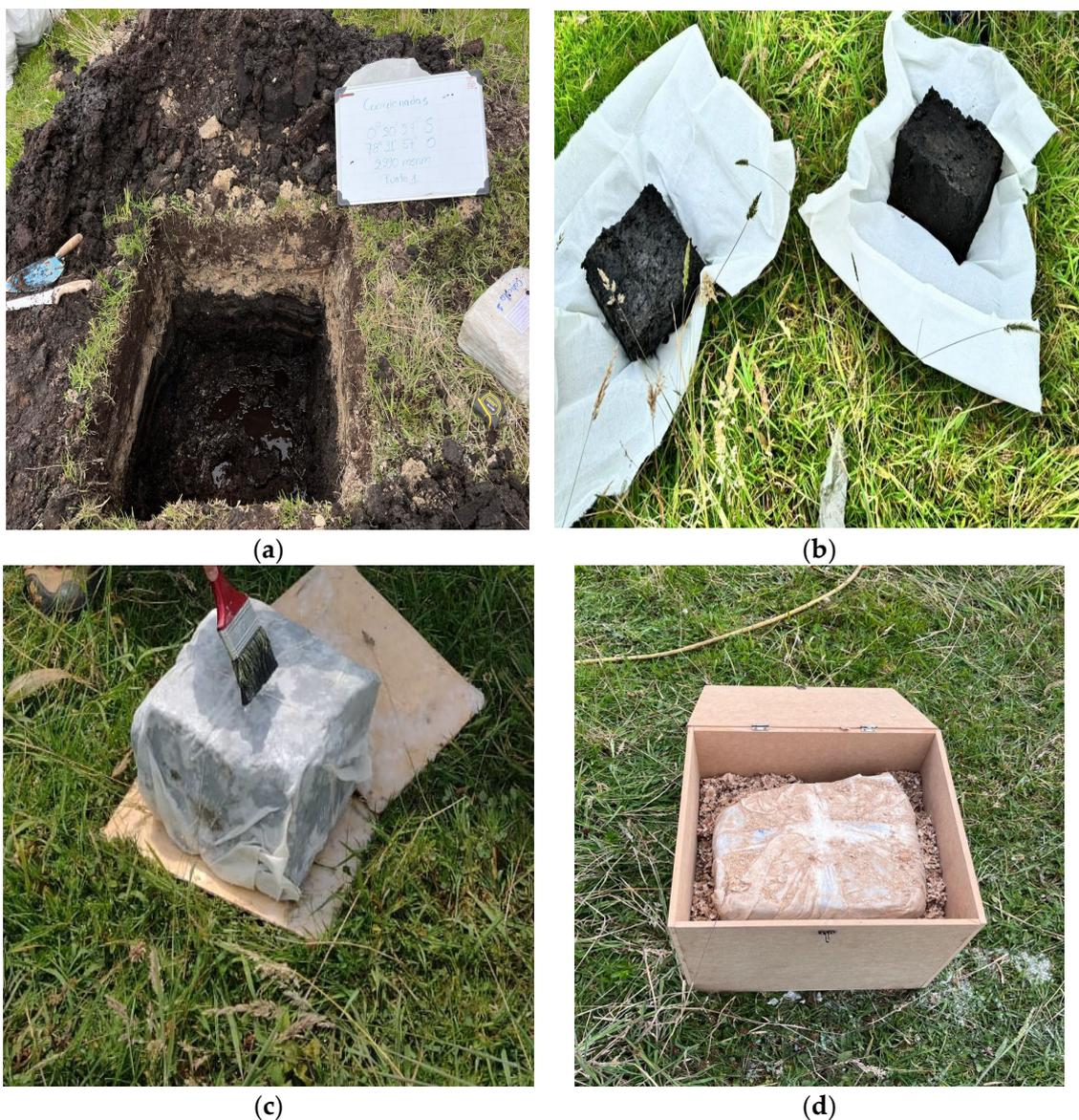
**Figure 2.** (a) Excavation of El Garrochal location; (b) placement of cheesecloth on samples; (c) placement of wax layer with cheesecloth to form three layers; and (d) samples placed in a wooden box for transport.
