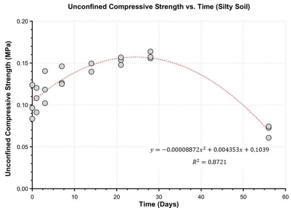
Figure 13. Correlation equation based on test results and elapsed time for unconfined compressive strength-silt.
