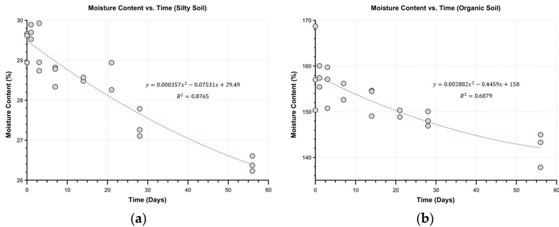
**Figure 11.** Correlation equation based on test results and elapsed time for the moisture content of (a) silt; (b) organic Soil.
