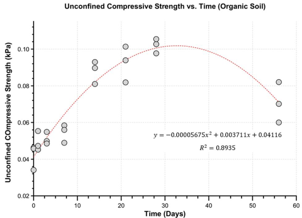
**Figure 14.** Correlation equation based on test results and elapsed time for unconfined compressive strength-organic soil.
