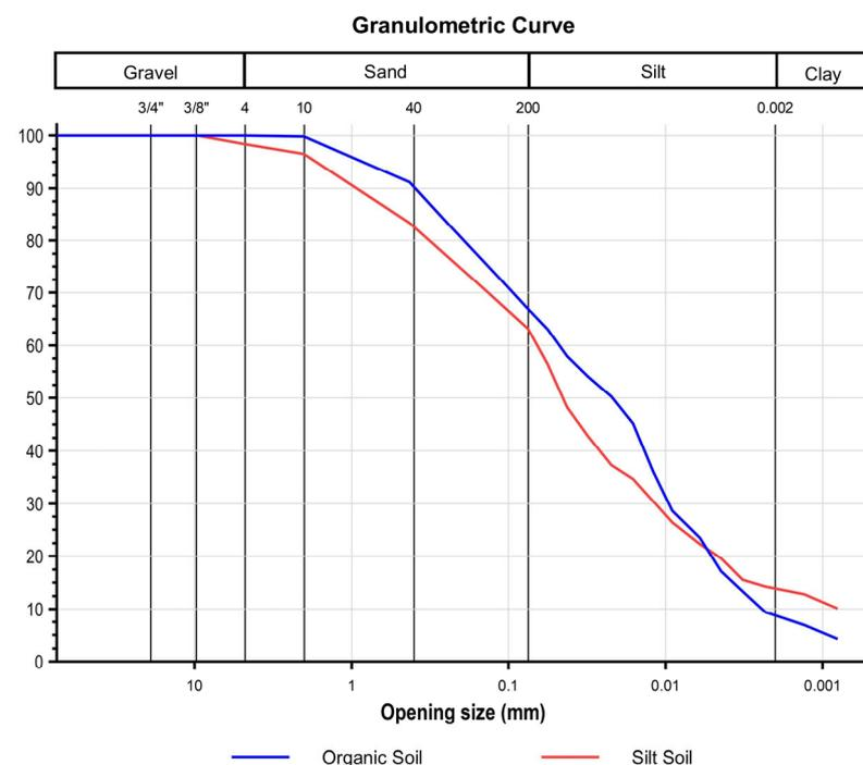
**Figure 5.** Granulometric curve (hydrometer), silt and organic soil.
