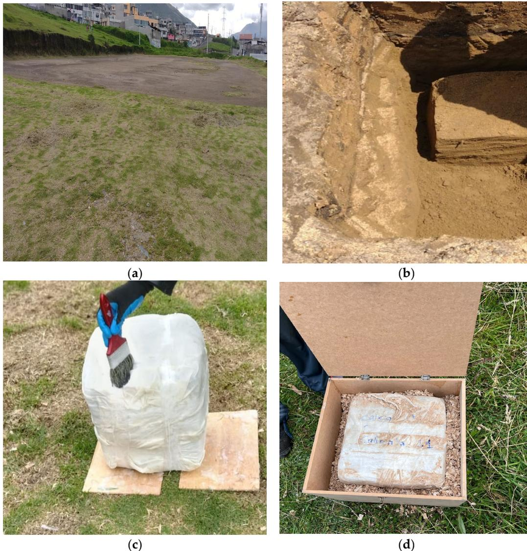
**Figure 3.** (a) Location of sampling point El Rocío-Guamaní; (b) sample extraction as intact blocks; (c) placement of a wax layer with cheesecloth to form three layers; and (d) sample placed in a wooden box for transport.
