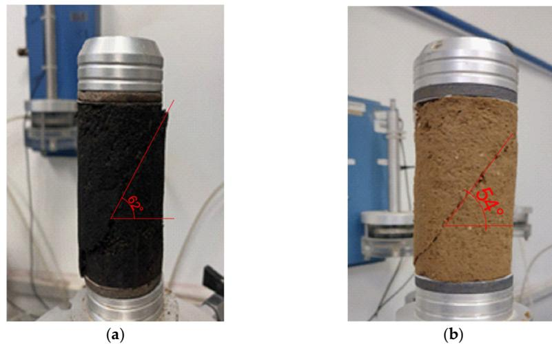
Figure 8. (a) Sample of organic soil tested; (b) sample of silt soil tested.
