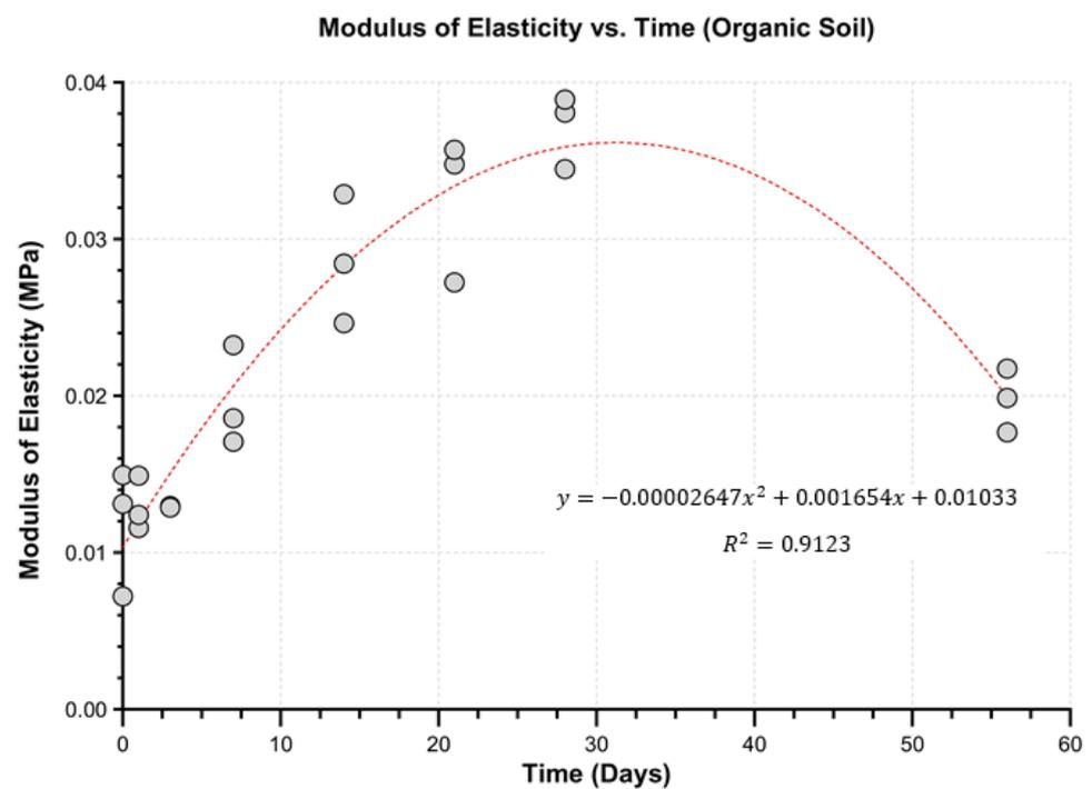
Figure 16. Correlation equation based on test results and elapsed time for the modulus of elasticity-organic soil.
