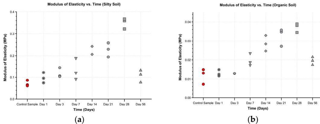
Figure 10. Modulus of elasticity. (a) Silt; (b) organic Soil.
