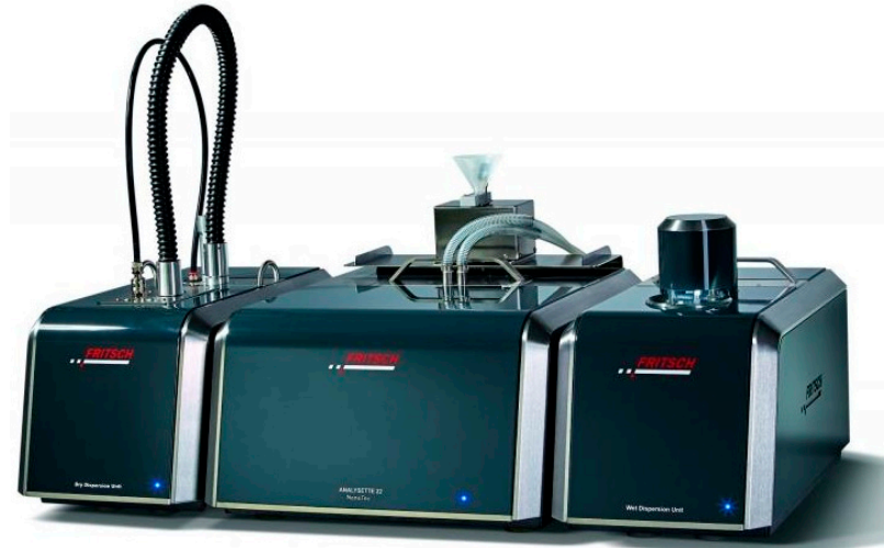
Figure 2. The Analysette 22 MicroTec plus laser diffractometer (right to left): wet dispersion unit, measuring unit and dry dispersion unit.
