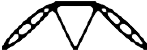
Figure 10. An optimal centrally loaded beam obtained by running the code provided by Ferrari et al. [47].
