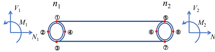
Figure 2. Stress sampling points for a 2D beam element.
