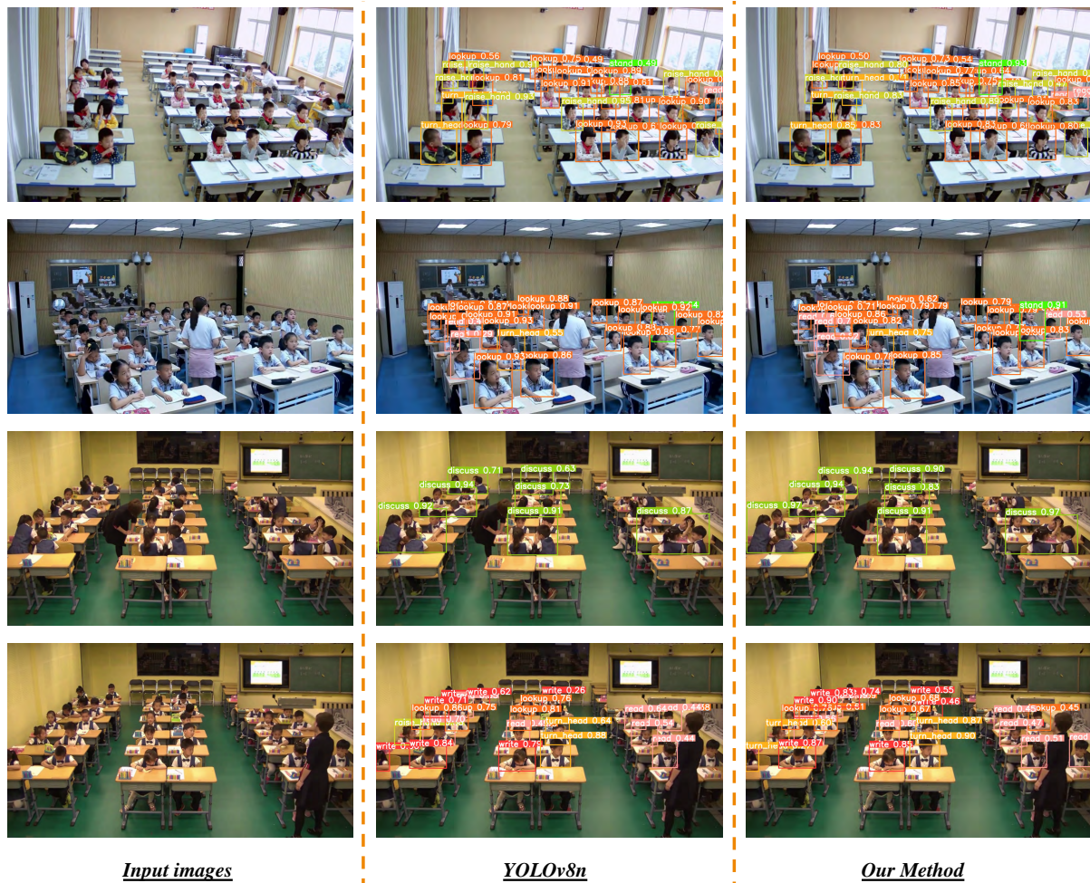
Figure 7. From left to right are the original image, the YOLOv8 detection image, and the SBD-Net detection image. We can intuitively observe that SBD-Net achieves better results while assigning more weights to the difficult samples, and it obtains better results.
