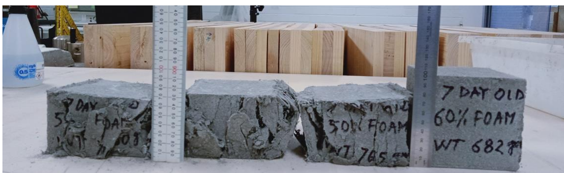
Figure 12. Failure modes after compression test (GP mix foam content 59%).
