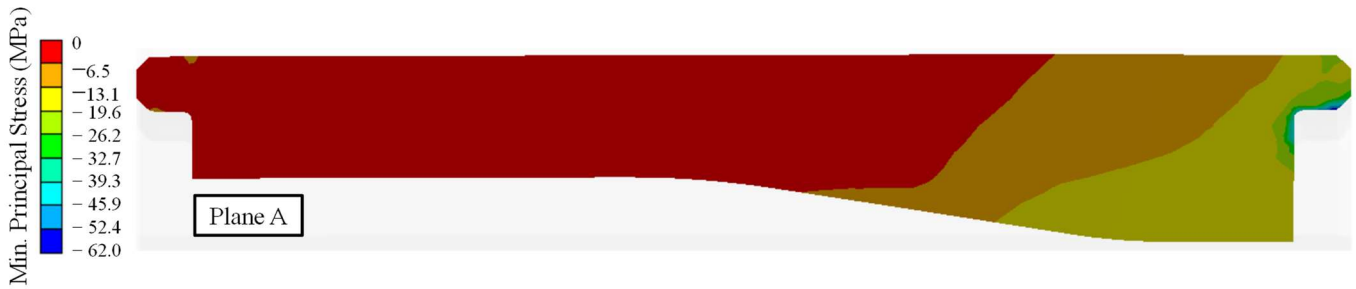
Figure 13. Minimum principal stress contours obtained from the 3D analysis in Plane A.
