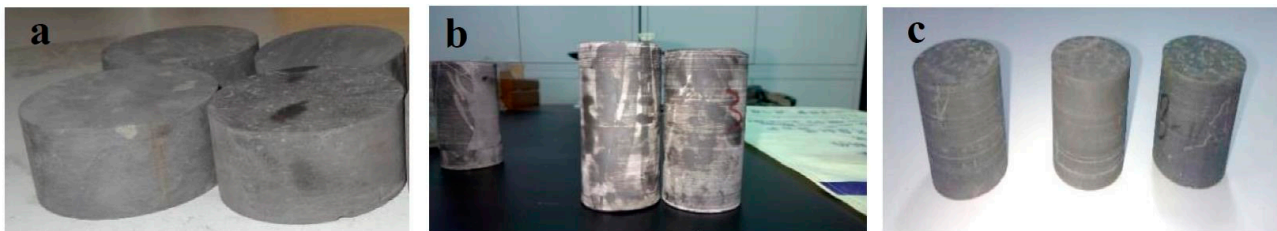
Figure 1. Examples of the specimens: (a) Brazilian splitting test, (b) uniaxial compression test, and (c) direct shear test.
