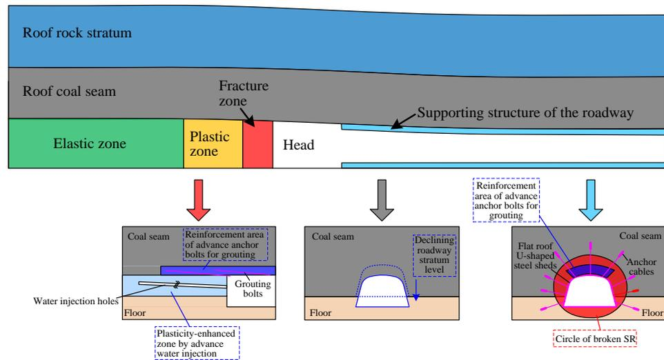
Figure 6. Schematic diagram of the synergistic support system of “LDAGF”.
