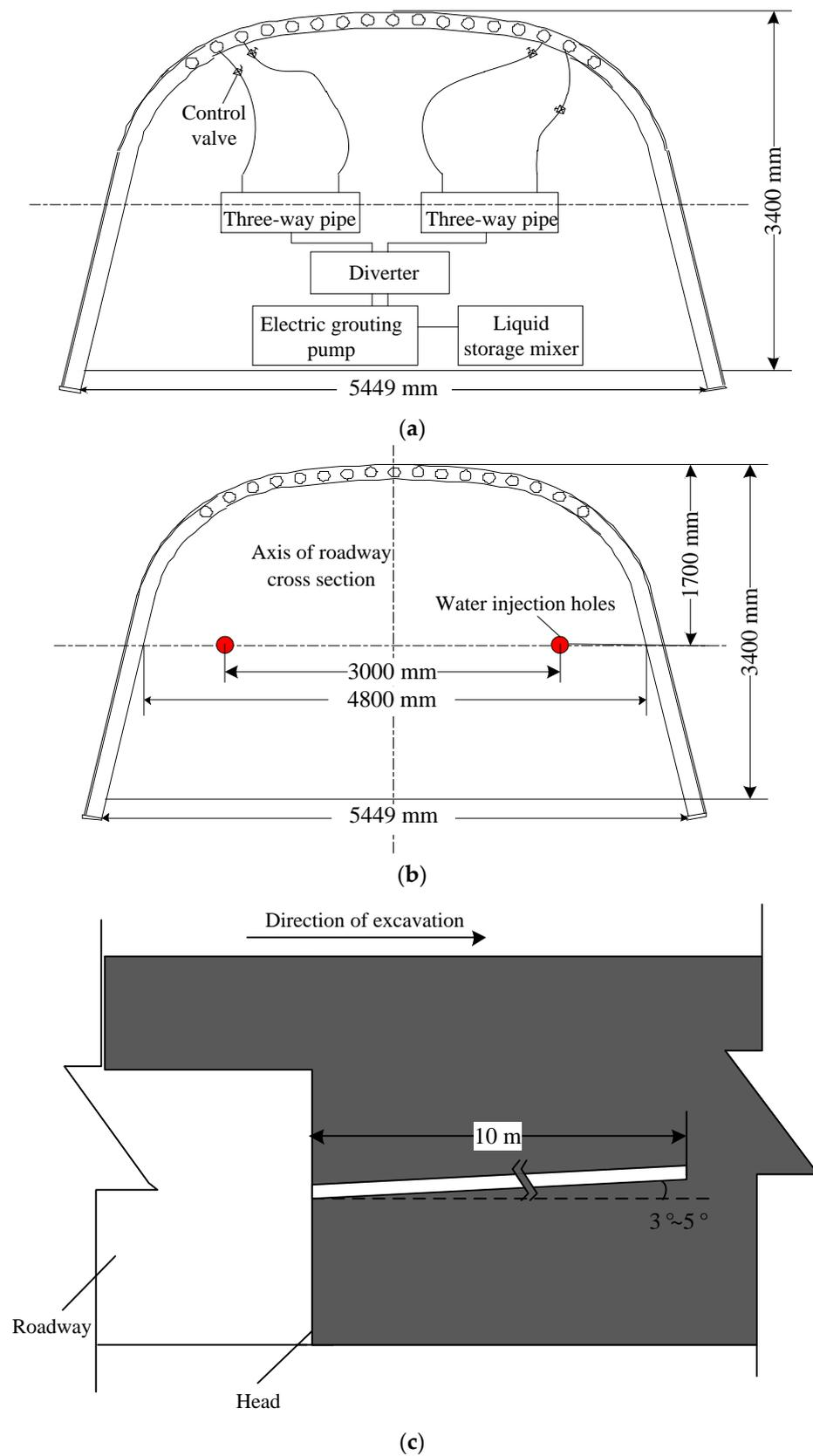
**Figure 10.** Layout of advance water injection and grouting in the roadway. (a) Layout of roadway advance grouting. (b) Section of the layout of advance water injection. (c) Cross section of the layout for the advance water injection.
