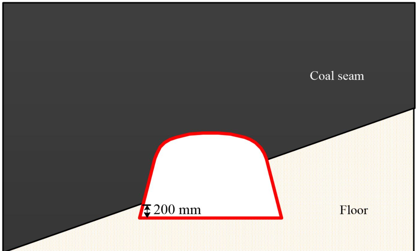
**Figure 8.** Schematic diagram of floor breaking and side lowering of the roadway.
