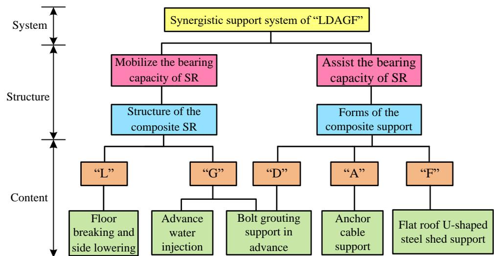
**Figure 5.** Basic components of the synergistic support system of “LDAGF”.
