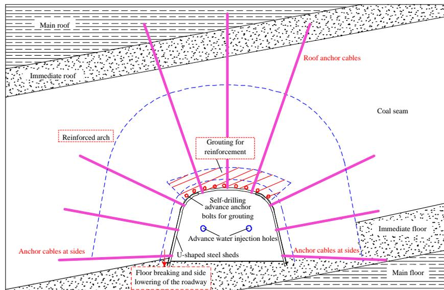
Figure 7. Synergistic support system of “LDAGF”.
