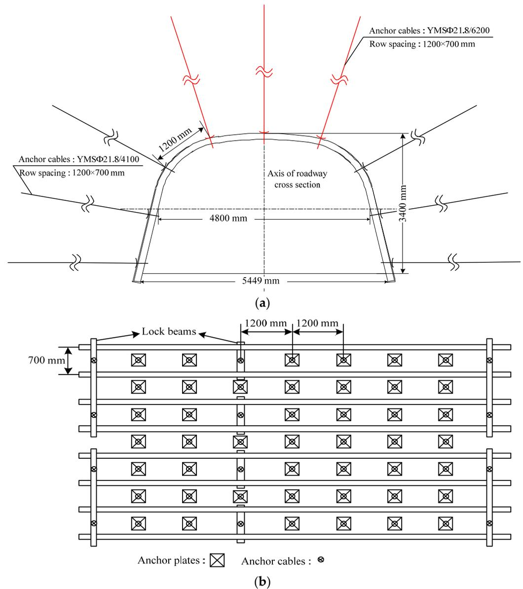
**Figure 11.** Schematic diagram of flat-roof U-shaped steel sheds and anchor cables for the roadway support. (a) Roadway section. (b) Roadway plan.
