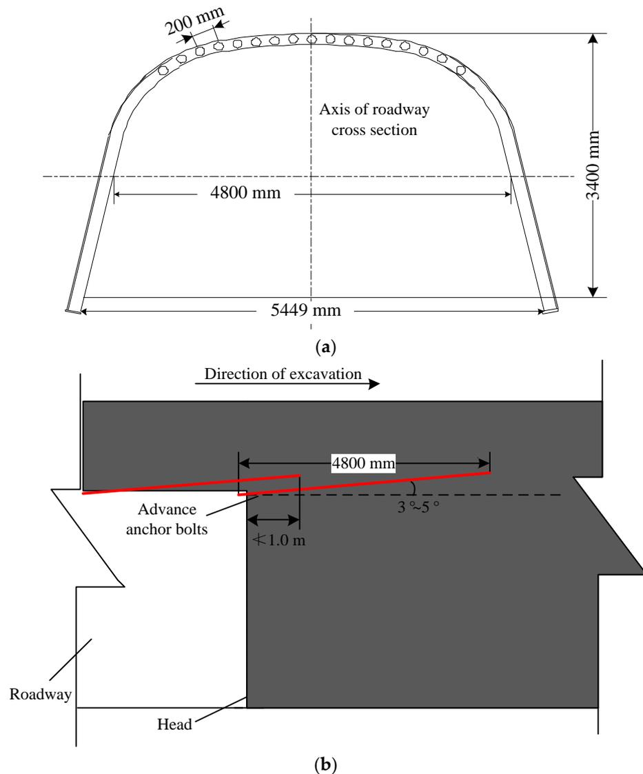
**Figure 9.** Layout of advance bolts in the roadway. (a) Roadway section. (b) Roadway cross section.
