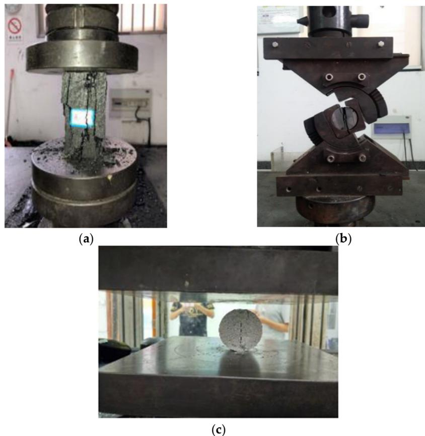
**Figure 3.** Mechanical experiments of coal and rock mass. (a) Uniaxial compression test (after experiment). (b) Shear test (after experiment). (c) Brazilian splitting test (after experiment).
