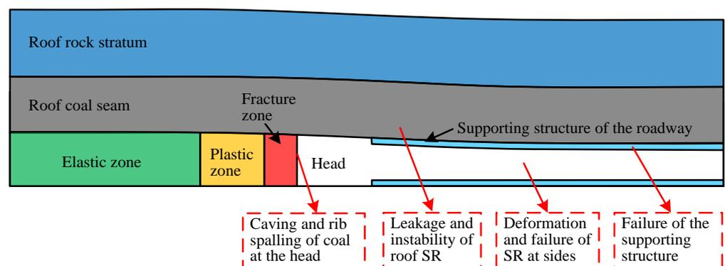
**Figure 4.** Structure diagram of SR in the ESFFMCFR.
