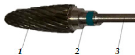
Figure 8. Conical-cylindrical dental bur: 1—dental bur active part; 2—dental bur neck; 3—dental bur foot.
