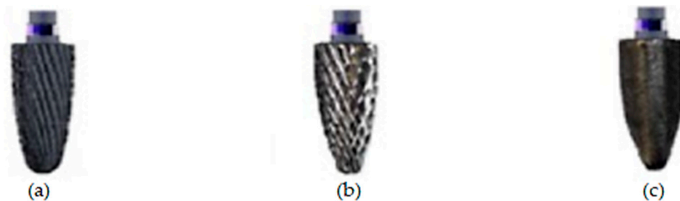
Figure 9. Methodology of establishing the circular crown mass of the dental bur active part: (a) specimen dental bur, after 1 h of operation; (b) worn dental bur after 4 h of operation; (c) dental bur with the circular crown of the active part, completely worn.
