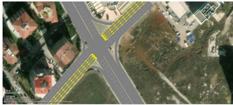
Figure 9. Treating the east-bound and west-bound directions as three-lane roads. Source: PTV VISSIM model.
