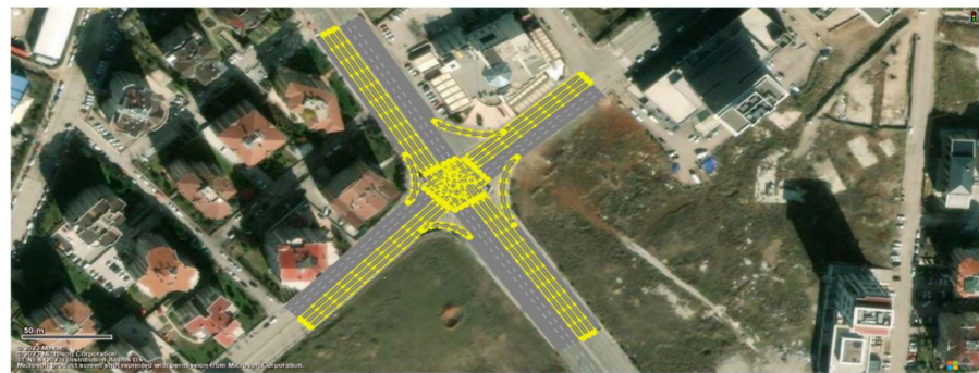
Figure 10. Intersection design calibrated for no lane changes: each lane as a separate link. Source: PTV VISSIM model.
