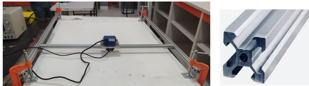
Figure 8. Structure for experimental validation (left) and detail of the aluminum profile (right).
