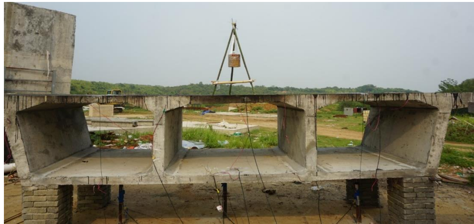
Figure 4. In situ arrangement of the explosion test.
