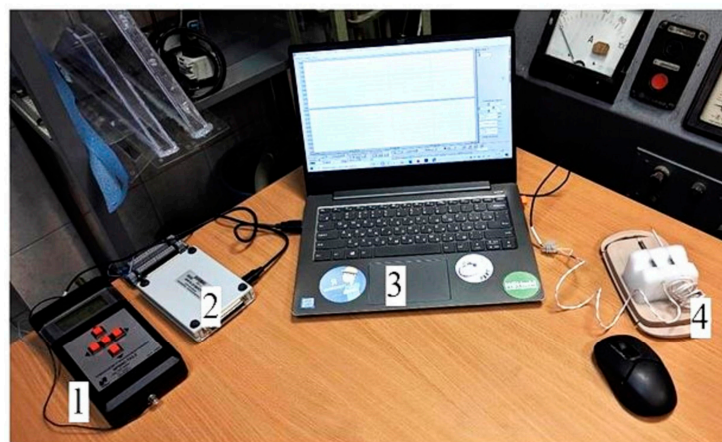
Figure 3. Main elements of measuring system based on thermal anemometry method: 1—constant-temperature hot-wire anemometer; 2—analogue-to-digital converter; 3—computer with specialized software; and 4—hot-wire anemometer sensors.
