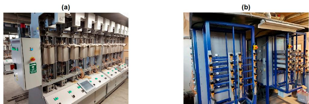
Figure 1. (a) One-sample creep test machines, (b) multi-sample creep test machines.
