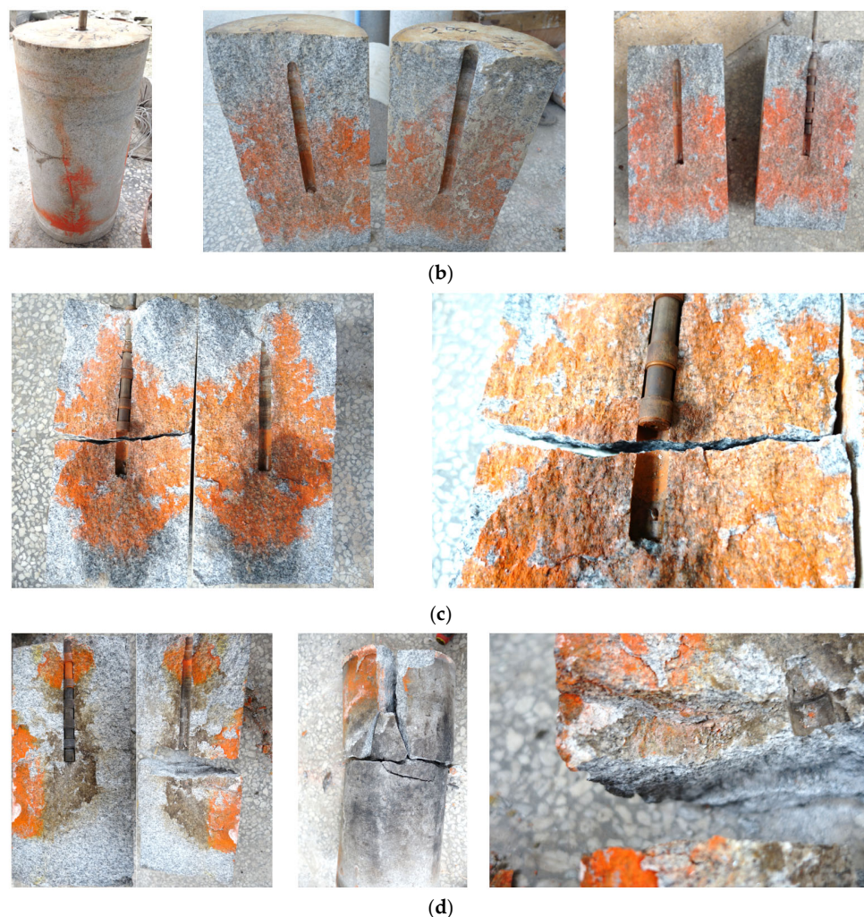
Figure 11. Hydraulic fractured granite rocks under high-temperature and high-pressure conditions. (a) Hydraulic fractured rocks at 100 °C; (b) hydraulic fractured rocks at 200 °C; (c) hydraulic fractured rocks at 300 °C; (d) Hydraulic fractured rocks at 400 °C.
