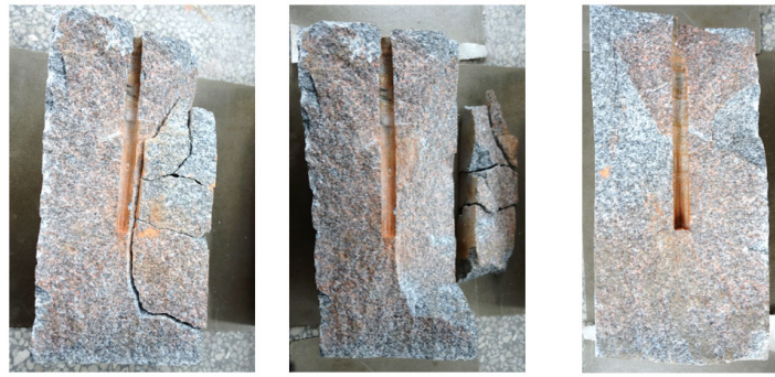
Figure 8. The final photos of hydraulic fractured rocks at room temperature.
