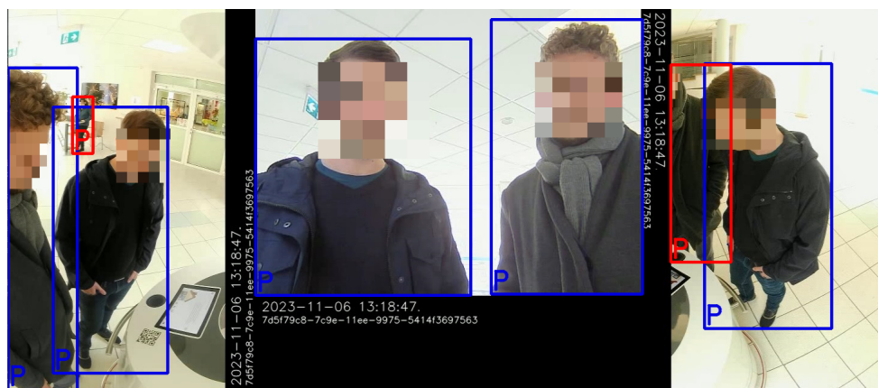
Figure 4. Detection of individuals at the city hall through multiple cameras evaluates engagement by examining the area of bounding boxes. Blue boxes represent engaged individuals, while red boxes signify either non-users or background objects. Exocentric camera outputs are shown in the left and right images, and the center video is from Furhat’s egocentric camera. Participant faces are anonymized to safeguard their privacy.
