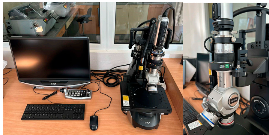
Figure 10. Digital 3D microscope used for angular positioning and evaluation of the cutting blade wear.
