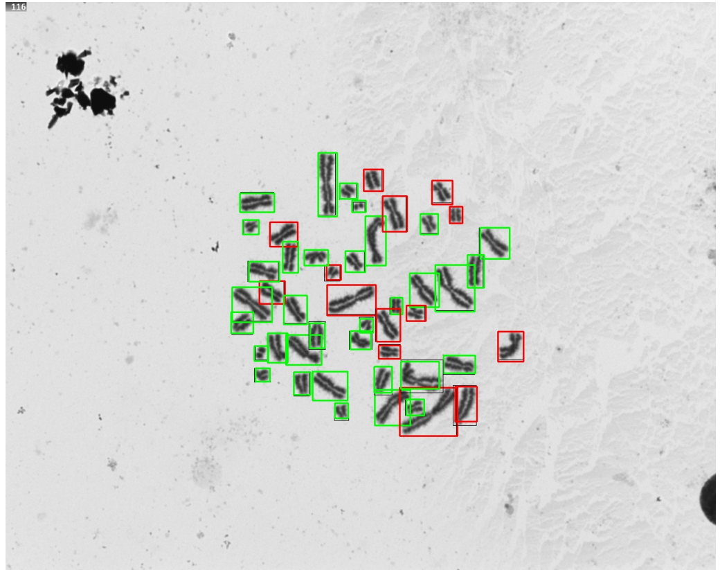
Figure 7. Prediction for the chromosomes of the image 2Gy-329 for the experiment where the Spline thresholding technique with 2 \times 2 closing filter was employed. In green: predictions as ‘non-dicentric’; in red: predictions as ‘dicentric’.
