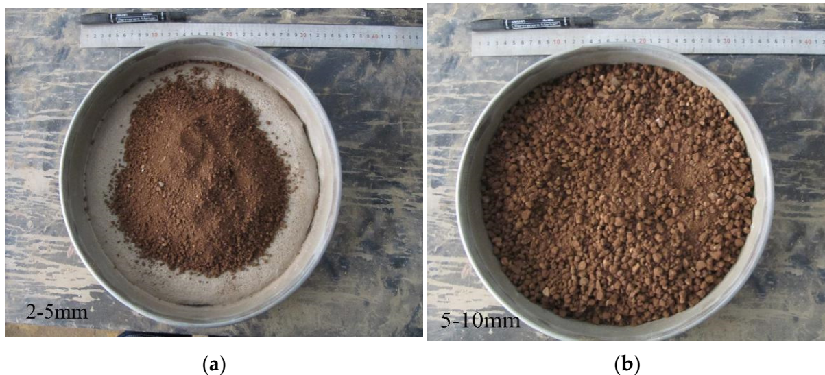
Figure 3. Rock blocks for uniaxial compression test with size of (a) 2–5 mm and (b) 5–10 mm.
