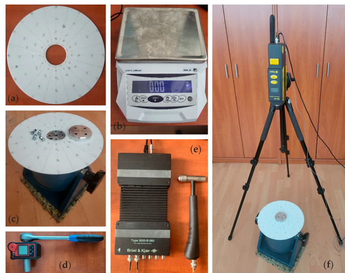
Figure 2. Experimental chain: (a) manufactured specimen; (b) digital balance; (c) unmounted specimen with the designed fixture put on the robust frame (modal shaker); (d) torque wrench with digital torque adaptor; (e) input module and modal hammer; (f) vibrometer with the specimen prepared for the analysis.
