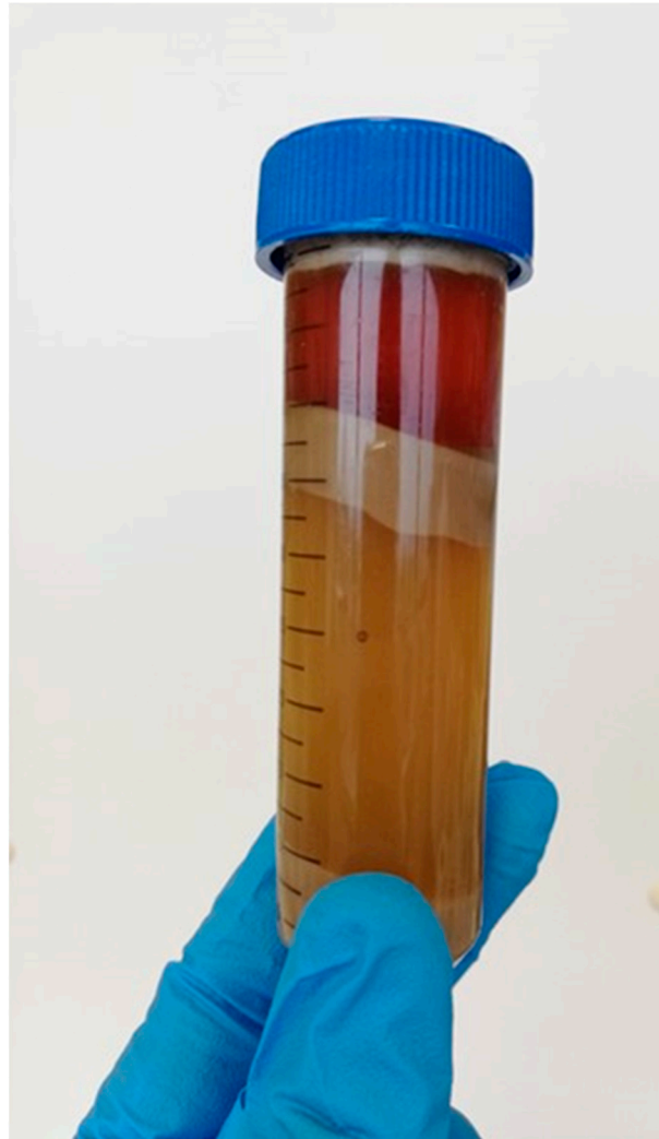
Figure 2. Fractions obtained after centrifugation ( 3000\times g , 10 min) of the silage of the hake viscera (from top to bottom: oil, floating interphase, liquid and pellet).
