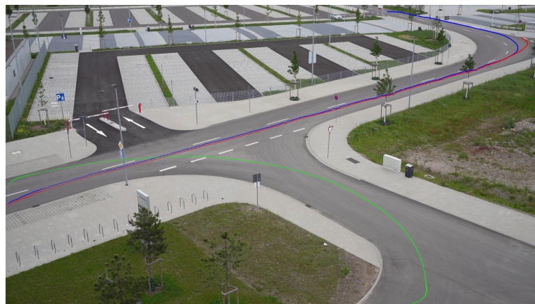
Figure 4. Original image of the T-junction with raw data of three different trajectories shown as blue, green, and red lines.
