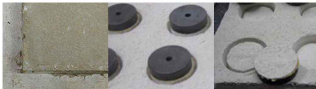
Figure 5. Reference concrete slabs prepared for pull-off testing with applied repair composite and cut-out specimens.
