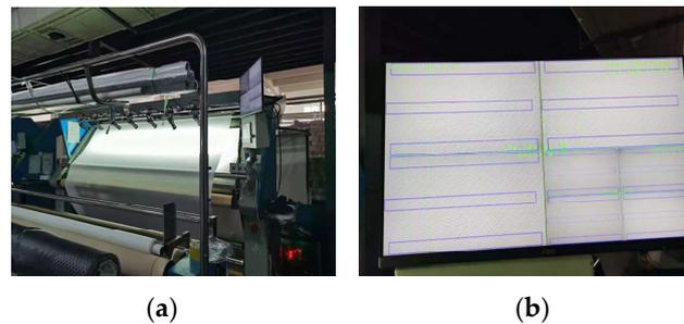
**Figure 12.** Fabric defect detection platform. (a) Defect detection system, (b) defect detection view.
