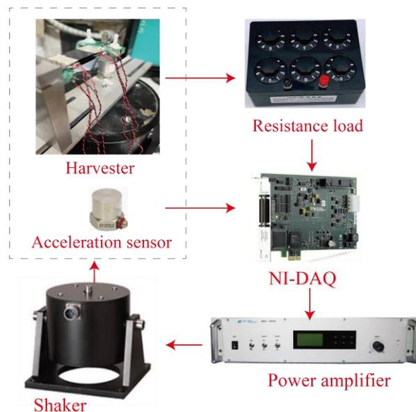
**Figure 3.** Experimental setup of the proposed PEH.
