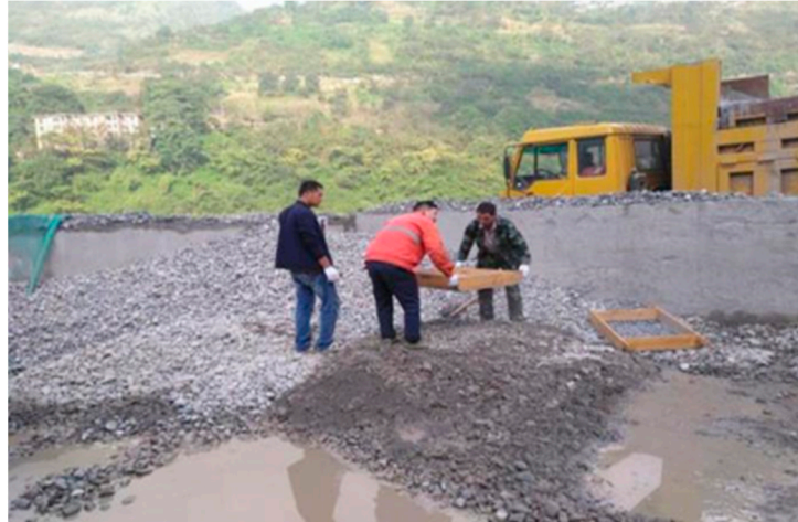
Figure A4. In situ aggregate sampling and gradation analysis.
