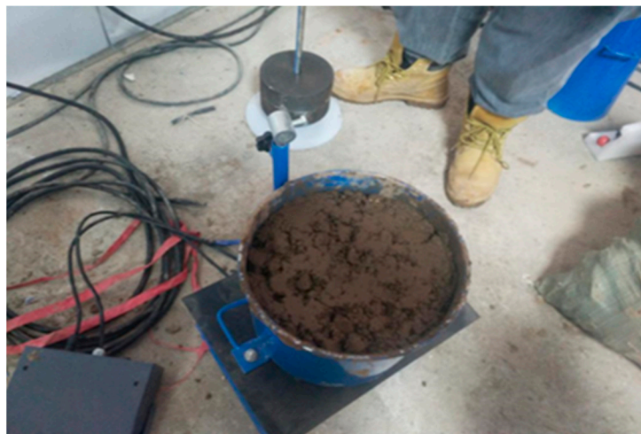
Figure A6. Workability test (VC test) using the Vebe apparatus.
