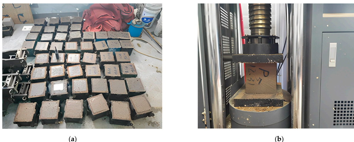
Figure 2. (a) Laboratory compressive strength test sample preparation. (b) Testing.
