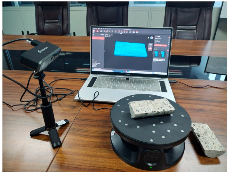
Figure 2. Fracture surface morphology reconstruction by three-dimensional laser scanning.
