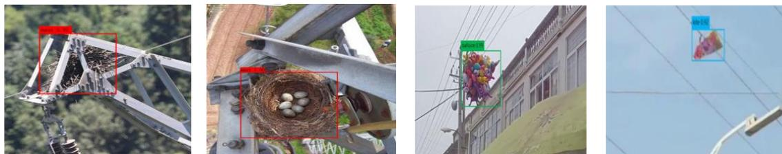
Figure 9. Example image of RCDAM-Net model detection.
