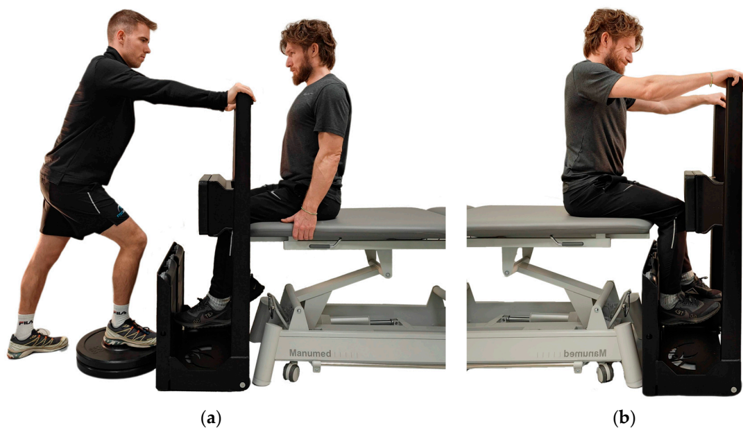
Figure 2. Experimental setup for the quadriceps strength test (Quad-H) and hamstring strength test (Ham-H) in the H-station. (a) General setup for the Quad-H test with a 25 kg weight plate and tester securing the H-station during testing. (b) General setup for the Ham-H test.
