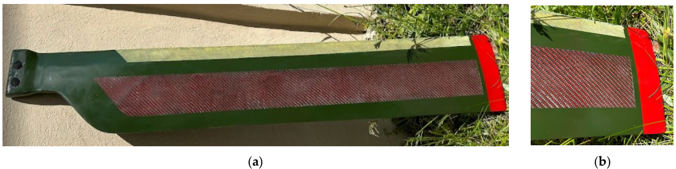
Figure 14. Composite blade/ (a) Final blade shape manufactured using 3D-printed mould. (b) Detail of blade tip area.
