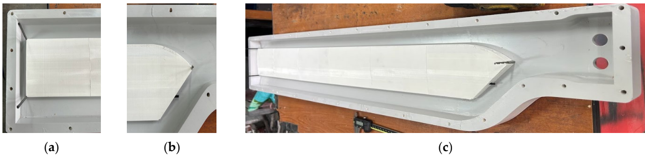
Figure 8. Centring the core in the mould. (a) Distal end. (b) Proximal end. (c) Lower mould-positioning of the blade core.
