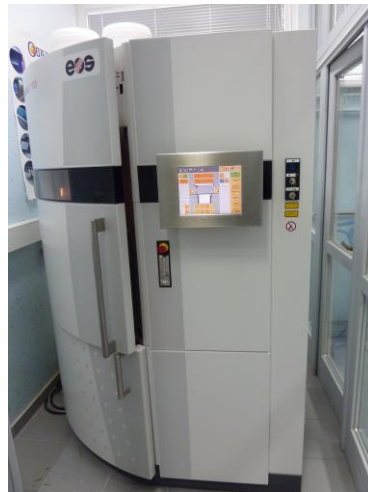
Figure 3. Formiga P100, a 3D printer on which test specimens are made.
