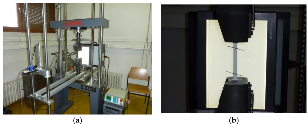
Figure 2. Testing of tensile properties: (a) universal testing machine Messphysik Beta 50-5 ; (b) testing the test specimen.
