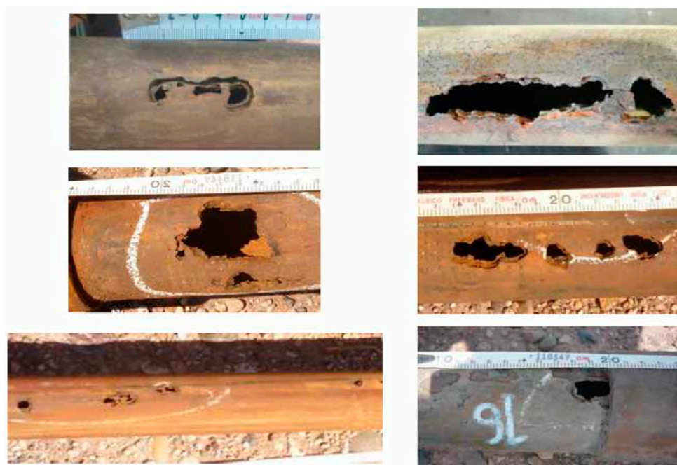
Figure 12. Tubing corrosion in the Vaca Muerta formation. Reprinted with permission from Ref. [80]. Copyright 2014, Society of Petroleum Engineers.
