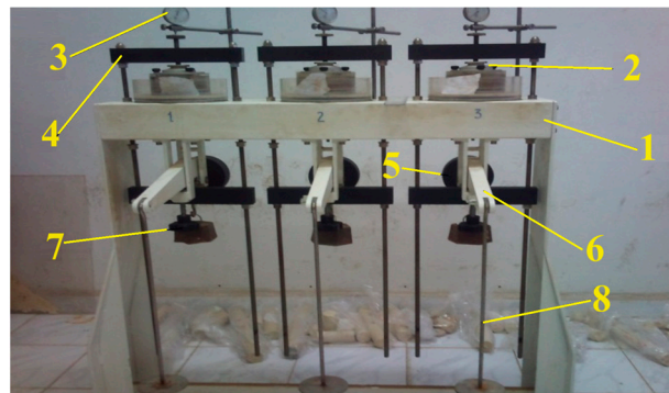
Figure 7. Consolidation test device (oedometer).
